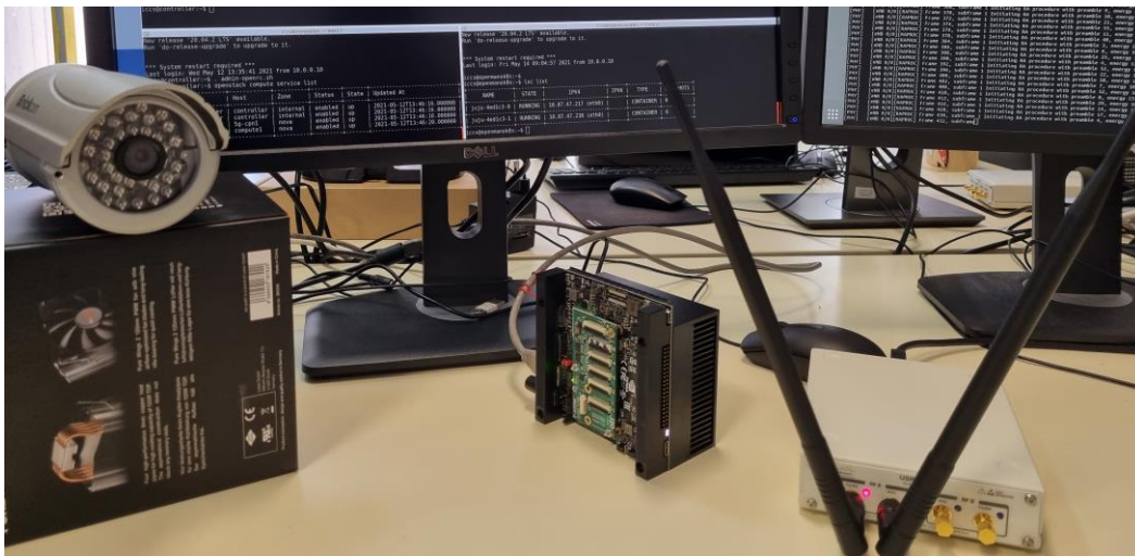
Figure 5: 5G-IoT device components.
